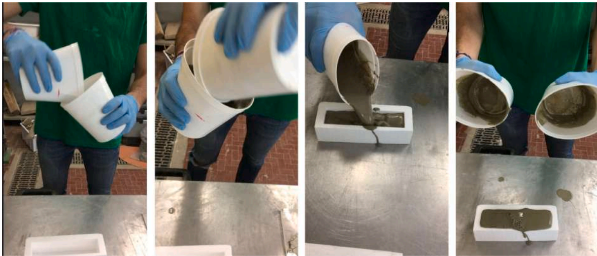
Fig. 1. Casting phase of a two-component grout sample according to the used procedure. From the left to the right: the component A is poured into the component B, the mixed grout is poured in the empty tank and after that the casting of the sample is carried out.
