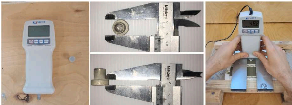
Fig. 5. Penetrometer used for the surface compression strength (SCS) assessment. Left: the used dynamometer. Centre: details of the flat circular bit (15.05 mm of diameter and 5 mm of thickness). Right: phase of the SCS assessment with the reading of F (N). Todaro et al. (2020) .
