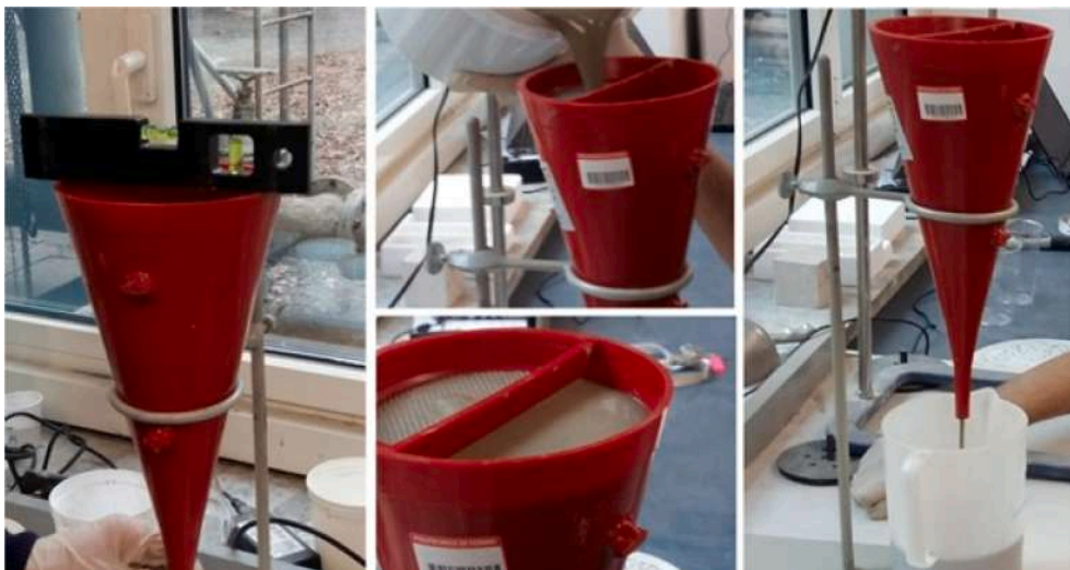
Fig. 3. Marsh funnel used for the viscosity assessment and main phases of the procedure. Left: leveling of the funnel. Centre: filling of the funnel (1.5 L) with the component A till the notch. Care must be taken to plug the exit hole. Right: removal of the plug and contemporary starting of the time record till the complete flow of 1 L. Todaro et al. (2019) .
