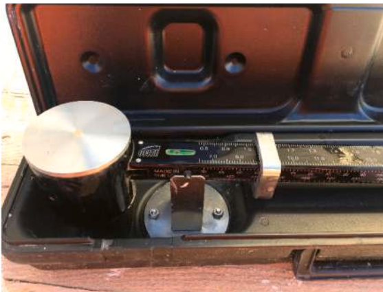
Fig. 2. Mud balance used for the unit weight assessment.
