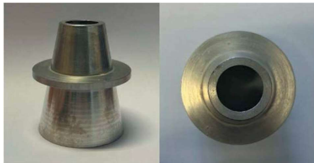
Figure 4. Mini flow cone front and from-above views.
