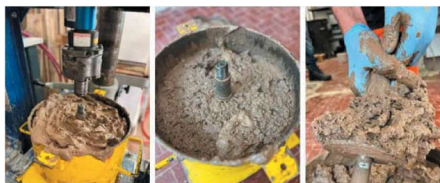
Figure 15. Dynamic adhesion test ID 1. Material completely poured into the steel container (left), material at the end of the test (right), extraction and visual analysis of the disc (right).
