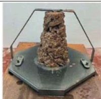
Figure 10. ID3 slump tests.
