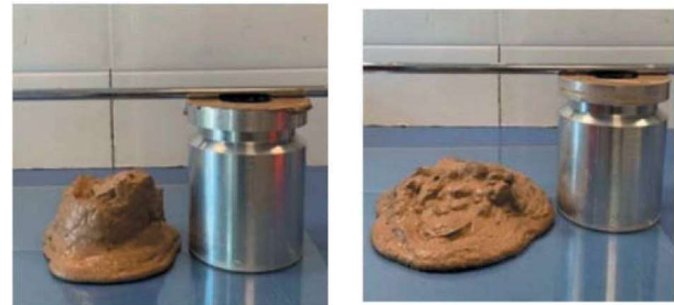
Figure 7. ID5 mini slump test pictures before jolting (left) and after (right).
