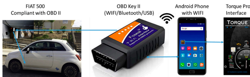
Figure 2. The trip data measuring scheme using OBD-key.
