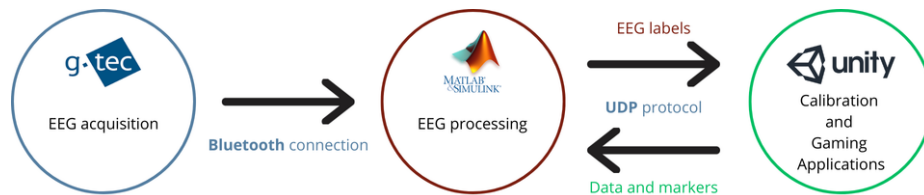
Fig. 1: Architecture of the self-paced brain-computer interface integrated with a virtual reality game.
