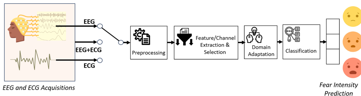
Fig. 6 Pipeline of the classification process involving EEG, ECG, or a combination of both. After the data has been preprocessed and segmented into epochs, suitable features are extracted, along with a channel
