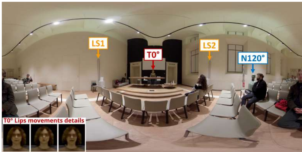
Figure 3: Equirectangular preview of the AV scene with lip movements as viewed from the listener's position. T_0^\circ indicates the target speaker, LS1 and LS2, the two loudspeakers, N_{120^\circ} the noise at 120^\circ azimuth represented by the dummy-head. In the low left corner, lip movements details are shown.
