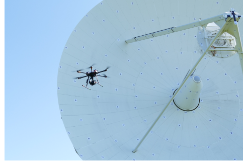
Fig. 2: Unmanned aerial vehicle in front of the prepared legacy 20 m VLBI radio telescope RTW at GOW, which is equipped with coded photogrammetric targets at the whole receiving unit.
