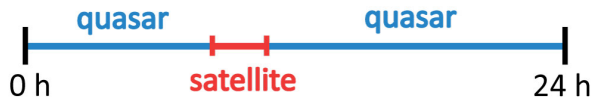
Fig. 3 Illustration of the scheduling approach. The schedule consists of a 40 minute period of satellite scans surrounded by quasar scans.
