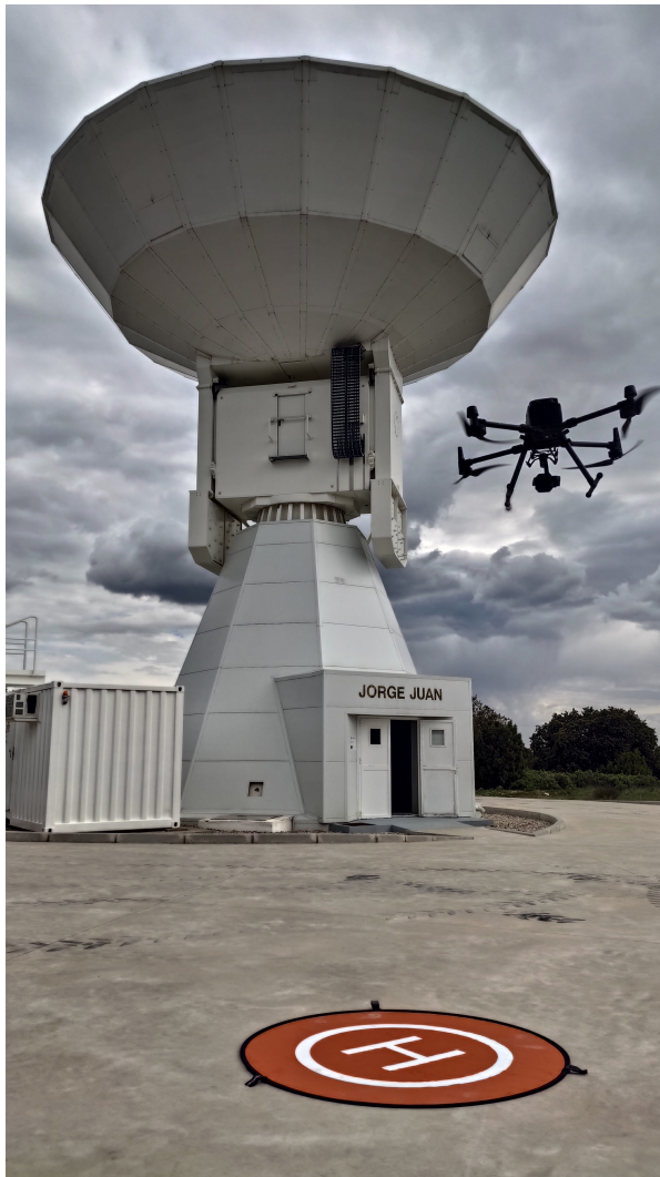
Fig. 2 Campaign for the measurement of the radio telescope deformations by using drones.
