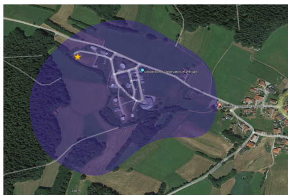
(1) LNA case exclusion zone (purple) and real location of DORIS (yellow star) at the Geodetic Observatory Wettzell
