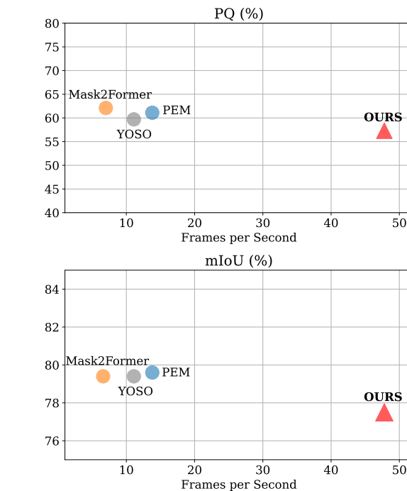
Figure 1. BiSeNetFormer delivers comparable or superior performance in comparison to existing methods while being the fastest multi-task architecture for image segmentation.
