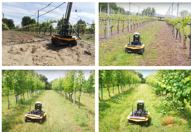
FIGURE 1. Field tests with the Jackal platform in different seasonal periods of the same crop. Lush vegetation and thick canopies reduce the GPS accuracy, affecting its reliability and the overall navigation pipeline. Our proposed segmentation-based algorithm exploits semantic segmentation properties to provide a proportional controller that drives the robotic platform along the whole row.
