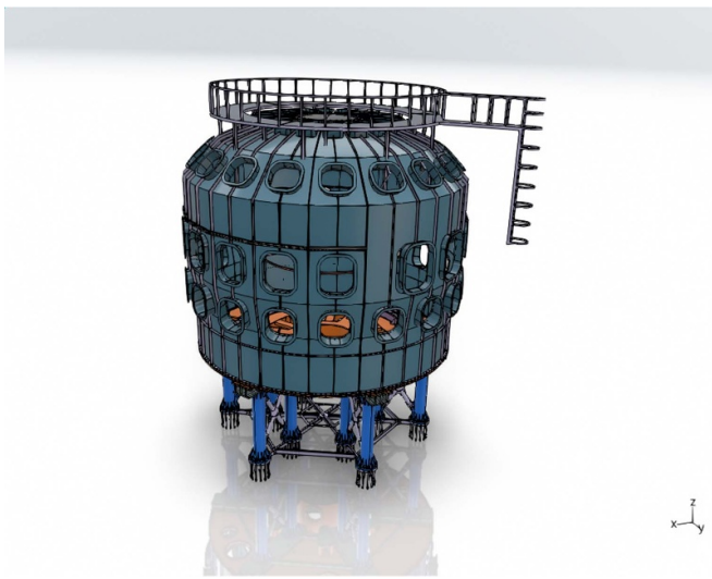
Figure 10. Render of the cryostat vessel and of the base structure. Reproduced with permission from DTT team.
