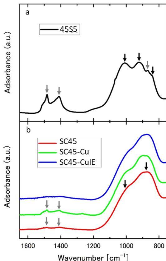
**Figure 6:** FT-IR spectra for 45S5 (black solid line), SC45 (red solid line), SC45-5Cu (green solid line), and SC45-CuIE (blue solid line). Adsorption peaks arising from SiO<sub>4</sub> tetrahedra and carbonate groups are indicated by black and grey arrows, respectively.
