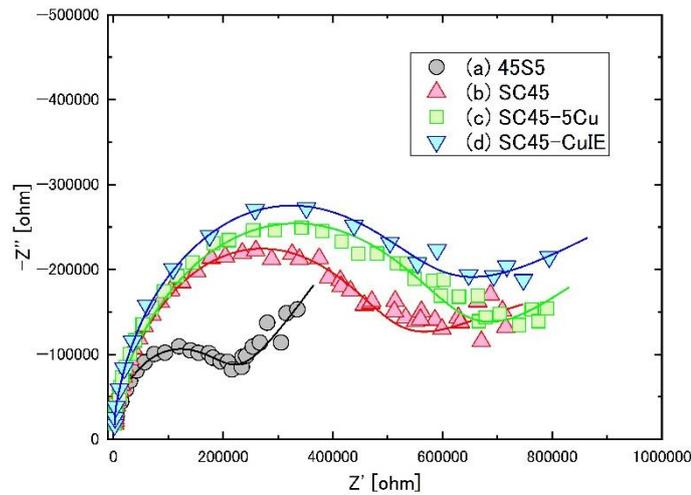
**Figure 3:** Nyquist plots for (a) 45S5 (black circles), (b) SC45 (red triangles), (c) SC45-5Cu (green squares), and (d) SC45-CuIE (blue inverse squares). The solid lines are the results of the fits employing two-equivalent circuit model.
