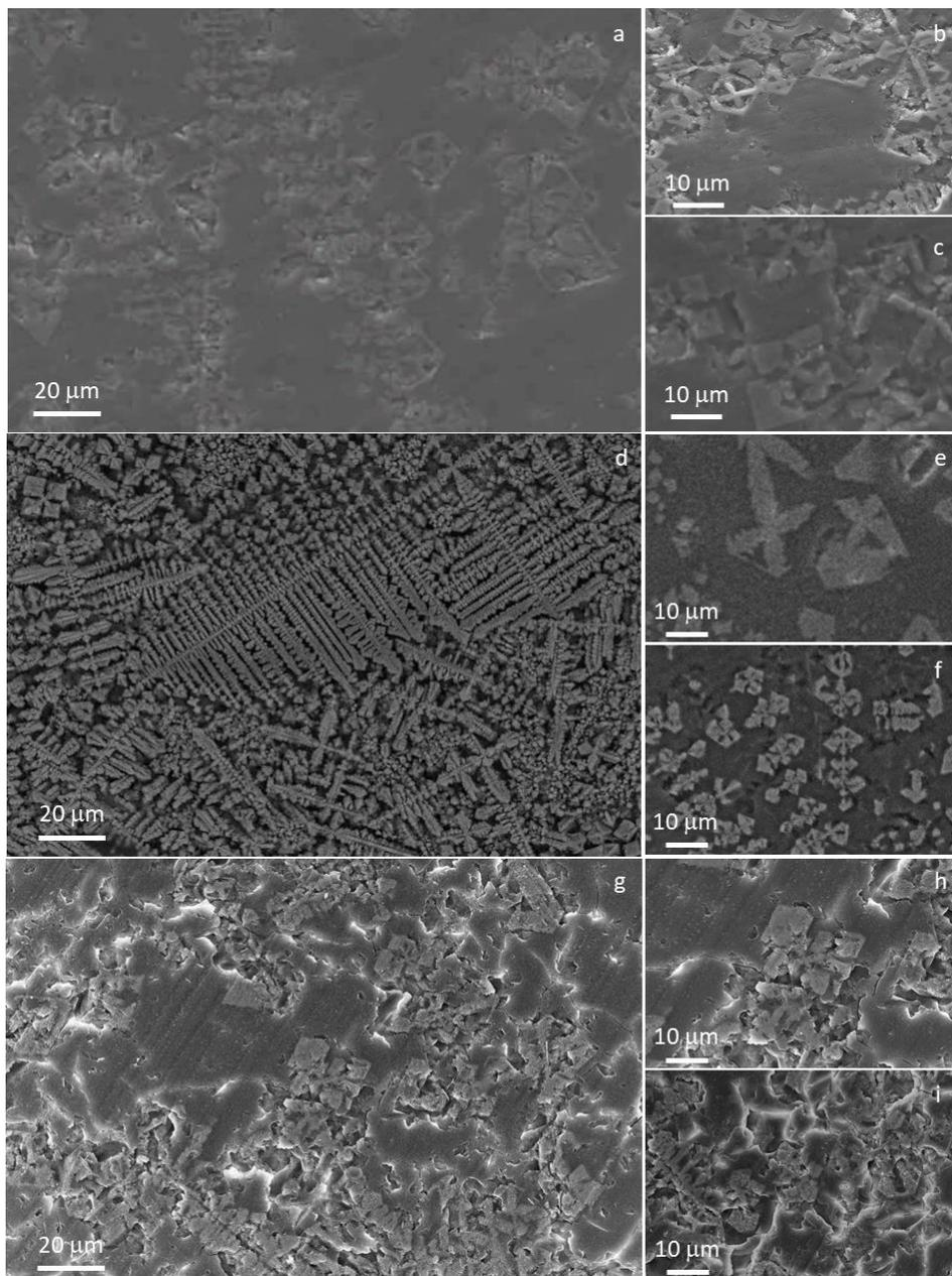
**Figure 1:** FE-SEM images of a SC45 a) magnification 2kx, b) and c) magnification 5kx; SC45-%Cu d) magnification 2kx, e) and f) magnification 5kx; SC45-CuIE g) magnification 2kx, h) and i) magnification 5kx.
