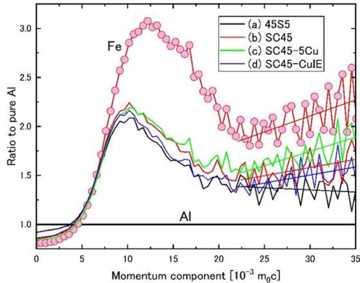
**Figure 4:** CDB spectra for (a) 45S5 (black solid line), (b) SC45 (red solid line), (c) SC45-5Cu (green solid line), and (d) SC45-CuIE (blue solid line) together with those of pure Al (Y=1) and Fe (red circles). All the spectra normalized to that of pure Al.
