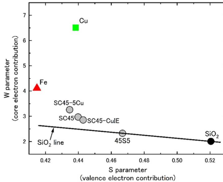
**Figure 5:** The correlation between S and W parameters taken from coincidence Doppler broadening spectra for 45S5, SC45, SC45-5Cu, and SC45-CuIE. All are plotted with black open circles. The data for SiO<sub>2</sub> (black solid circles) together with those for pure Fe (red solid triangles) and pure Cu (green solid squares) are presented for comparison. The solid line with the data of SiO<sub>2</sub>, denoted as the SiO<sub>2</sub> line, is drawn for guiding the eye.
