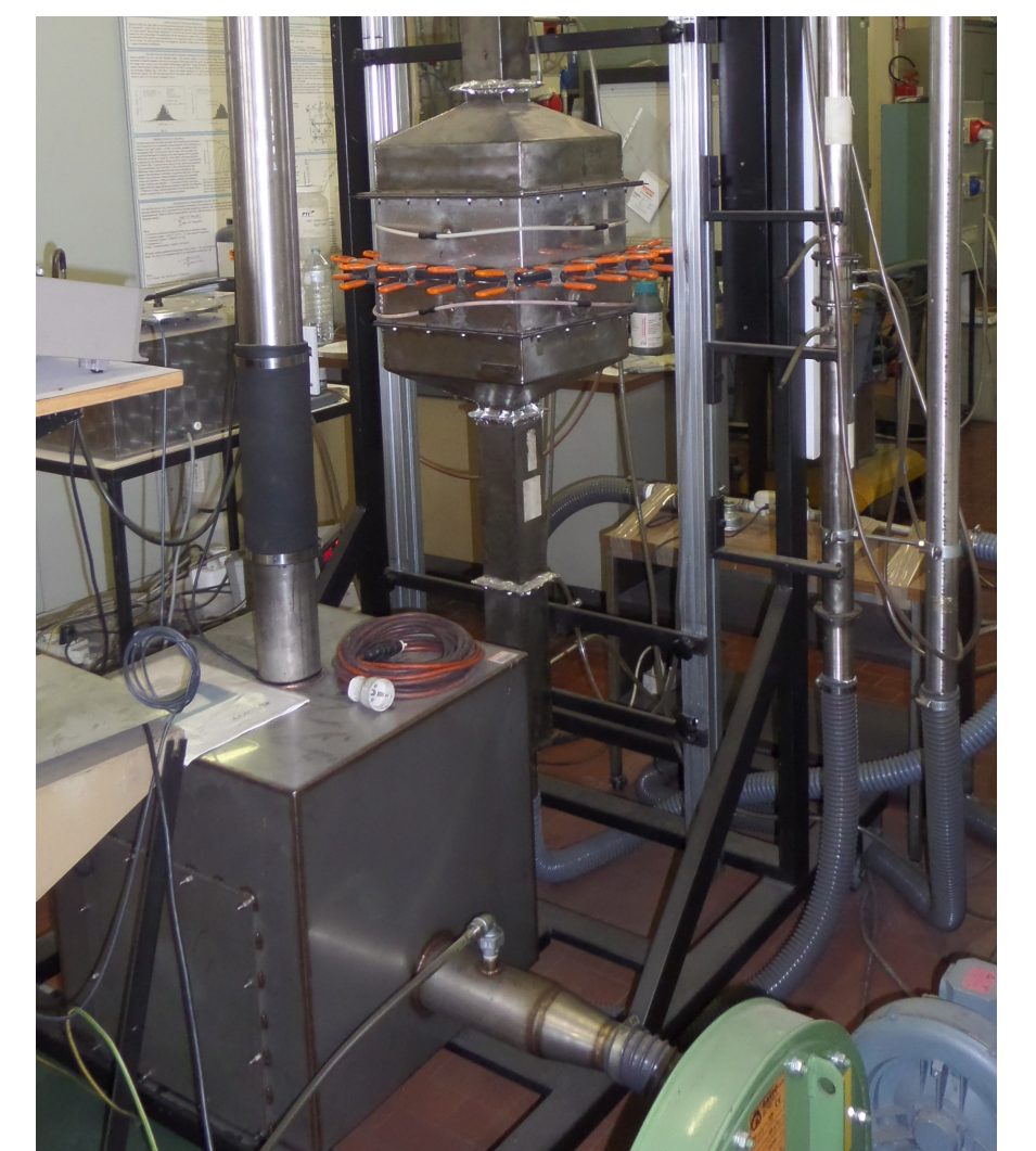
Figure 4. Filter media test rig.
