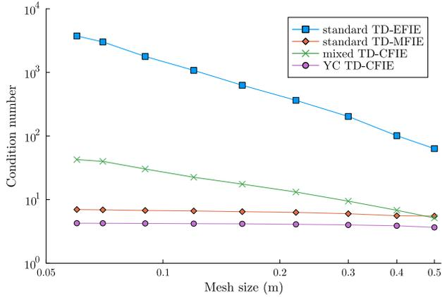
Fig. 6. Condition number of the matrix  $\mathbf{L}_0$  with respect to different mesh sizes of a cuboid of dimensions  $0.5\text{m} \times 2\text{m} \times 2\text{m}$ , obtained using different formulations. The time step is fixed at  $\Delta t = 3.33\text{ns}$ . The TD-EFIE and the mixed TD-CFIE exhibit dense discretization breakdown, whereas the TD-MFIE and the Yukawa-Calderón TD-CFIE do not.
