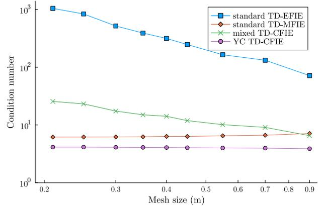
Fig. 8. Condition number of the matrix  $\mathbf{L}_0$  with respect to different mesh sizes of a torus with large radius  $3\text{m}$  and small radius  $1\text{m}$ , obtained using different formulations. The time step is fixed at  $\Delta t = 6.67\text{ns}$ . The TD-MFIE and the Yukawa-Calderón TD-CFIE do not suffer from dense discretization breakdown.
