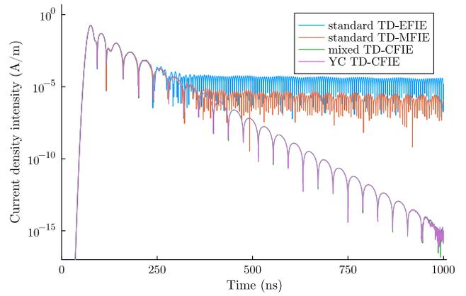
Fig. 7. Induced surface current density on a torus with two radii  $3\text{m}$  and  $1\text{m}$  at the point  $(x, y, z) = (-2.326, -1.885, -0.692)\text{m}$ , obtained using different formulations. The average mesh size  $h = 0.6\text{m}$ , and the time step  $\Delta t = 0.333\text{ns}$ . The TD-EFIE and TD-MFIE suffer from resonant instability. The TD-MFIE is also affected by the nontrivial nullspace of the static MFIE operator. The TD-CFIEs are resonant-free, but slowly decay.
