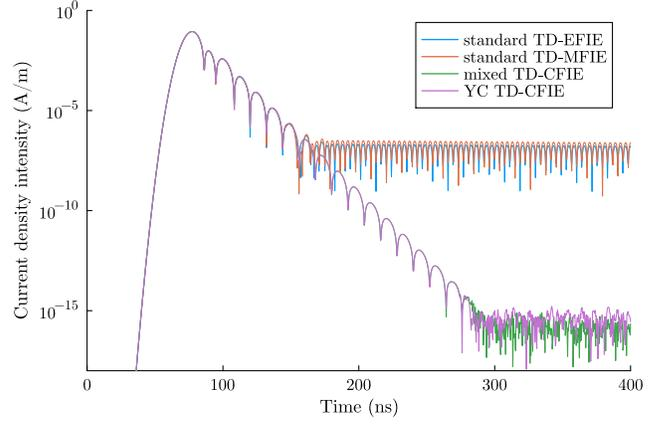
Fig. 3. Induced surface current density intensity on a sphere of radius 1m at the point  $(x, y, z) = (-0.534, -0.523, -0.644)\text{m}$ , obtained using different formulations. The average mesh size  $h = 0.3\text{m}$ , and the time step  $\Delta t = 0.333\text{ns}$ . The TD-EFIE and TD-MFIE suffer from resonant instability, whereas the TD-CFIEs do not.
