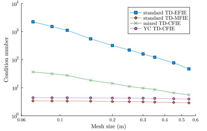
Fig. 4. Condition number of the matrix  $\mathbf{L}_0$  with respect to different mesh sizes of a sphere with radius 1m, obtained using different formulations. The time step is fixed at  $\Delta t = 3.33\text{ns}$ . The TD-MFIE and the Yukawa-Calderón TD-CFIE stay well-conditioned when the mesh size decreases.
