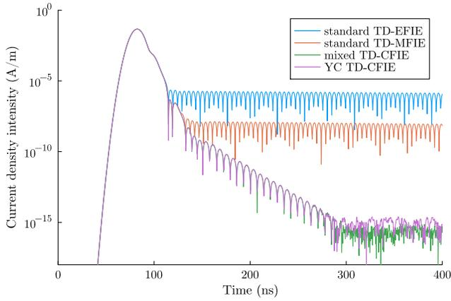
Fig. 5. Induced surface current density intensity on a cuboid of dimensions  $0.5\text{m} \times 2\text{m} \times 2\text{m}$  at the point  $(x, y, z) = (-0.25, -0.502, 0.761)\text{m}$ , obtained using different formulations. The average mesh size  $h = 0.15\text{m}$ , and the time step  $\Delta t = 0.333\text{ns}$ . The TD-EFIE and TD-MFIE suffer from resonant instability, whereas the TD-CFIEs do not.
