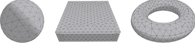
Fig. 2. Triangle mesh of different geometries used in numerical experiments. *Left*: a sphere with radius 1m discretized by 476 triangles. *Middle*: a cuboid of dimensions  $0.5\text{m} \times 2\text{m} \times 2\text{m}$  discretized by 1428 triangles. *Right*: a torus with two radii 3m and 1m discretized into 952 triangles.
