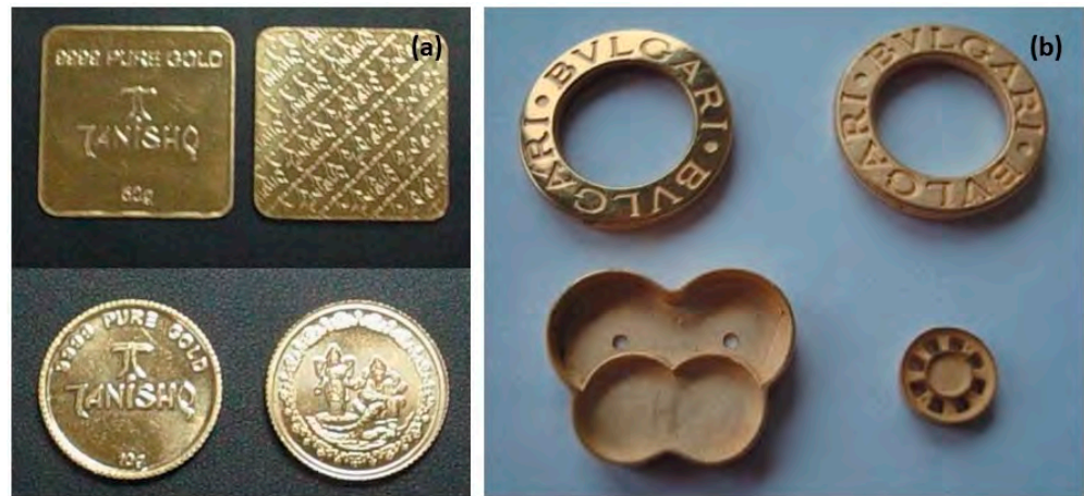
Figure 7. (a) Press and sinter of Tanishq pure gold coins by Titan, (b) MIM-produced 18-karat gold 3N pieces, Reprinted from ref. [19].
