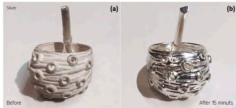
Figure 42. Electro-mechanical polished sample (a) before and (b) after a 15-min treatment, Reprinted from ref. [94].
