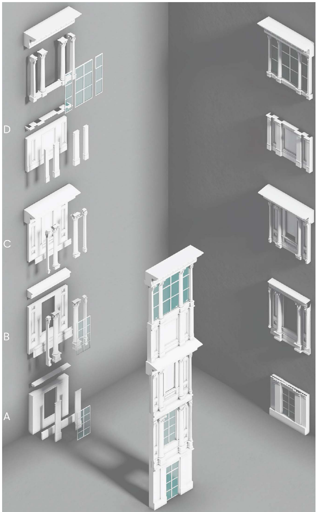
Fig. 7. "Dynamic model" of a part of the façade on five levels with an exploded view of the sub-components. Elaboration by L. Torresi.
