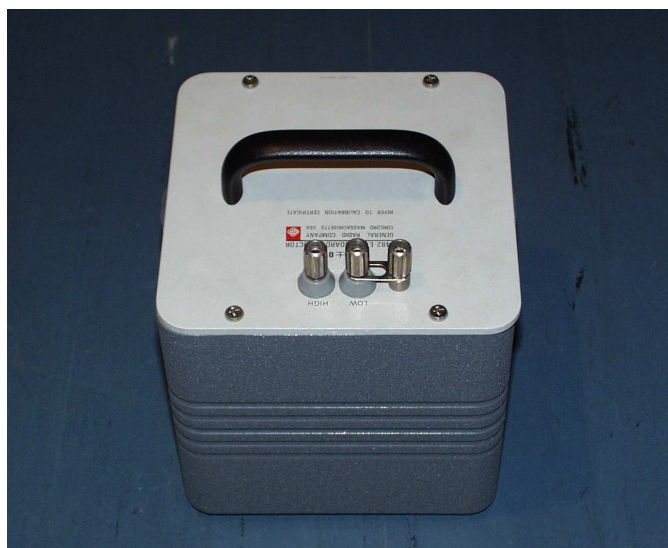
Fig. 1. General Radio 1482 toroidal inductance standard, configured as a two-terminal impedance.
