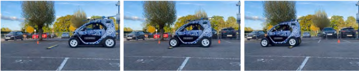
Fig. 26. Frames of the ZEBRA vehicle captured during the speed bump test.
