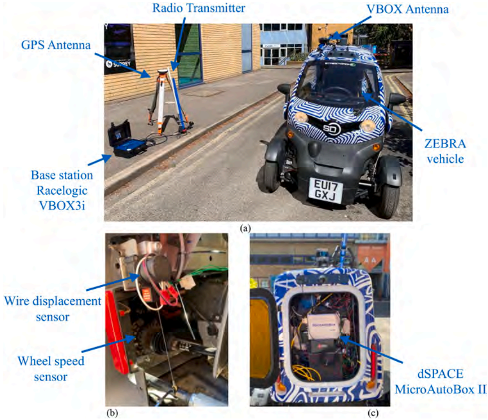
Fig. 24. (a) The ZEBRA vehicle of the University of Surrey equipped with a Racelogic VBOX3i dual GPS system; (b) wire suspension displacement and wheel speed sensors installed at the rear-left corner; and (c) the dSPACE MicroAutoBox II rapid control prototyping unit of the vehicle.
