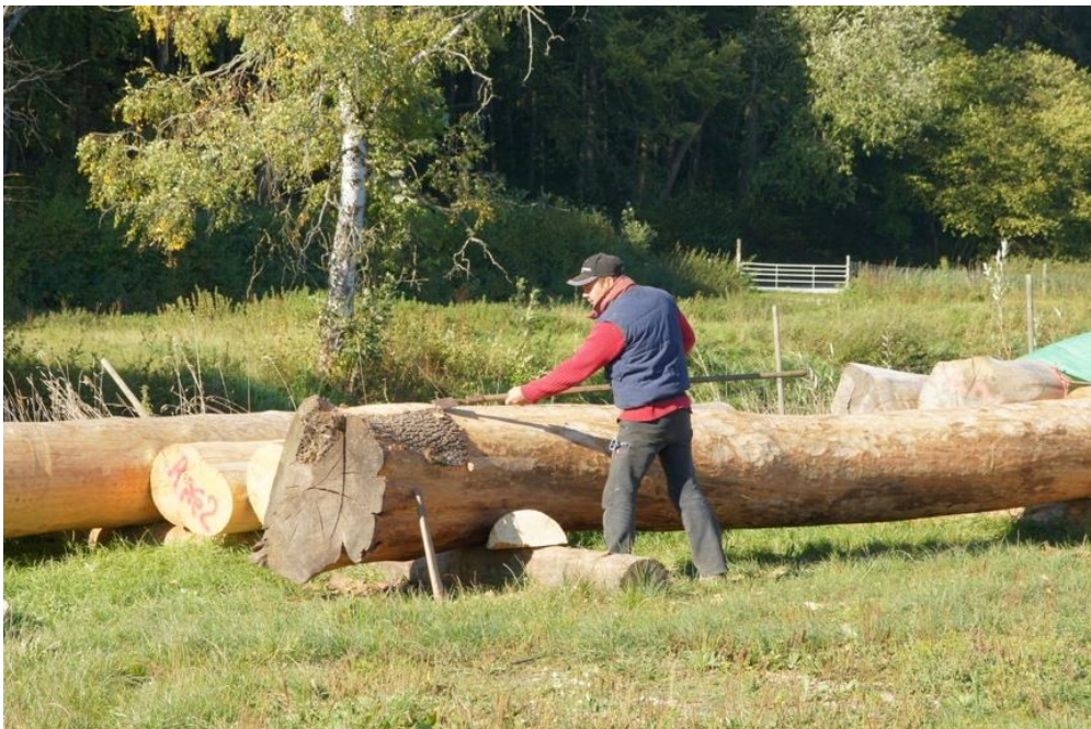
Figure 13. Manual debarking of wooden logs at the Biotal site. Source: Biotal Hofgemeinschaft blog, 2015
