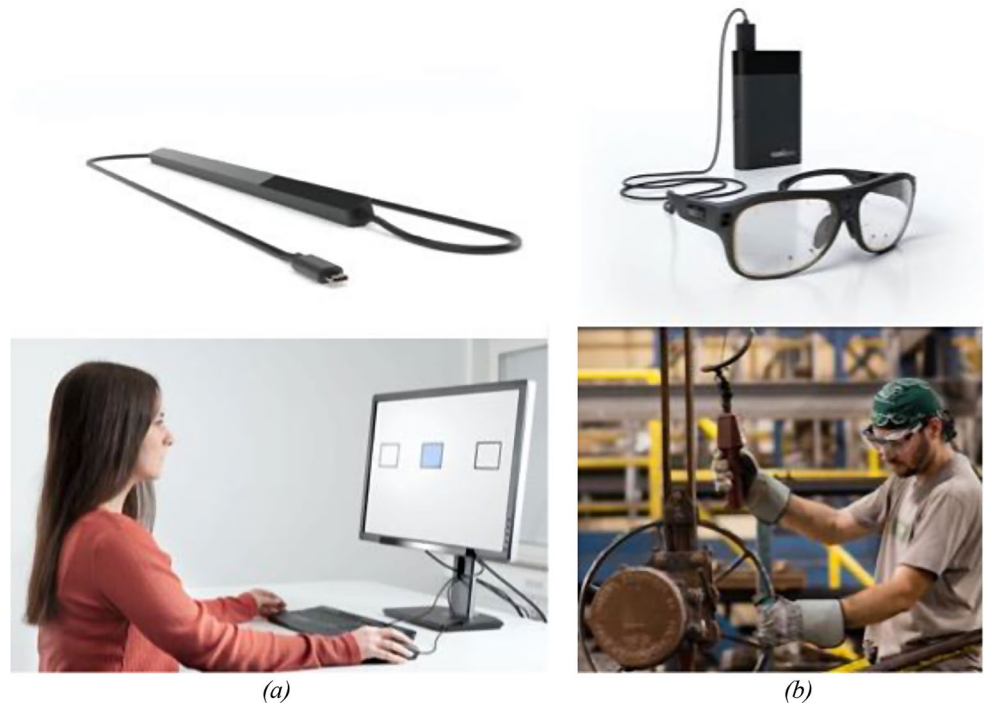
Fig. 2 Examples of VOG eye-trackers: (a) the screen-based Tobii Pro Fusion and (b) the wearable Tobii Pro Glasses 3 [14]
