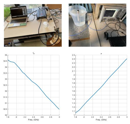
**Figure 5.** System to measure the dielectric constant of the tissue-like liquid (**top left**), and the quasiin vitro configuration (**top right**). Measured relative dielectric constant (**bottom left**) and conductivity S/m (**bottom right**).
