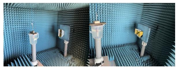
**Figure 6.** RP measurement set-up for the embedded antenna: cross-polarization (**left**) and co-polarization (**right**) components.
