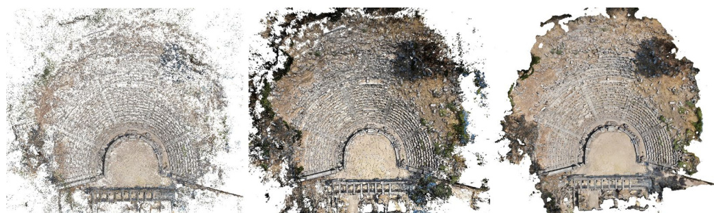
Figure 5. Images of the post-processing of data for the Theater. From the left, the alignment of cameras (1,256,561 points), dense cloud (261,238,304 points), and textured mesh (43,646,219 faces and 21,831,522 vertices). (E.C.G.).
