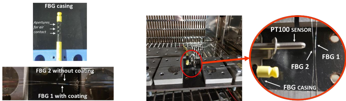
Figure 2 Sensors placed in the climatic chamber (on the left) and details about their set-up (on the right)
