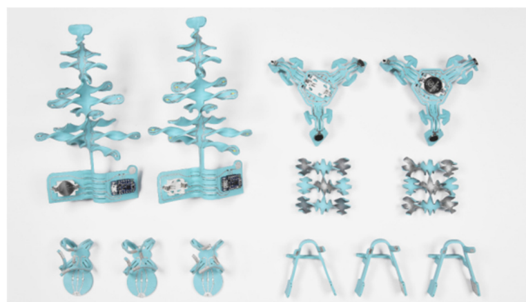
Figure 6. Self-folding conformable electronics FFF printed. Used with permission from Association for Computing Machinery, permission conveyed through Copyright Clearance Center, Inc. 2020 [22].
