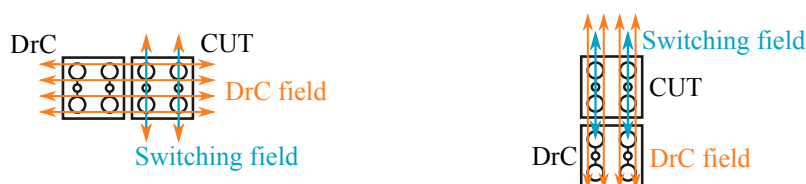
Fig. 3.5 Comparison between the direction of the switching field and the field generated by the DrC in adjacent horizontal and vertical cell-to-cell interaction.
