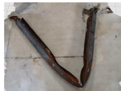
Figure 1(b). Deformed steel post
