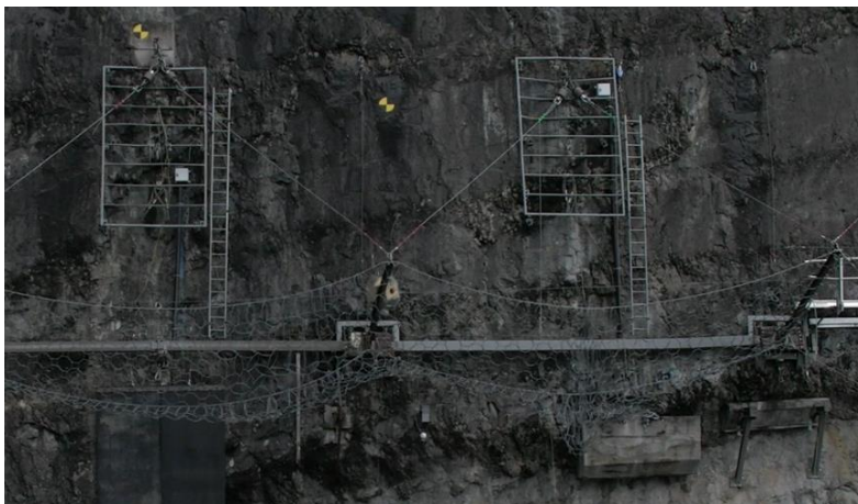
Figure 1(a). SEL impact on a 500 kJ flexible rockfall barrier steel
