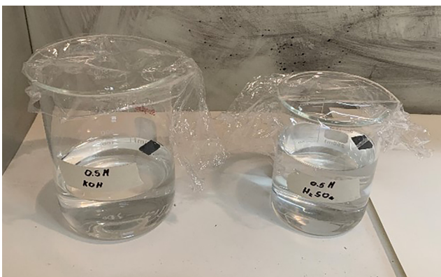
Figure 11 Experimental setup for the corrosive tests
