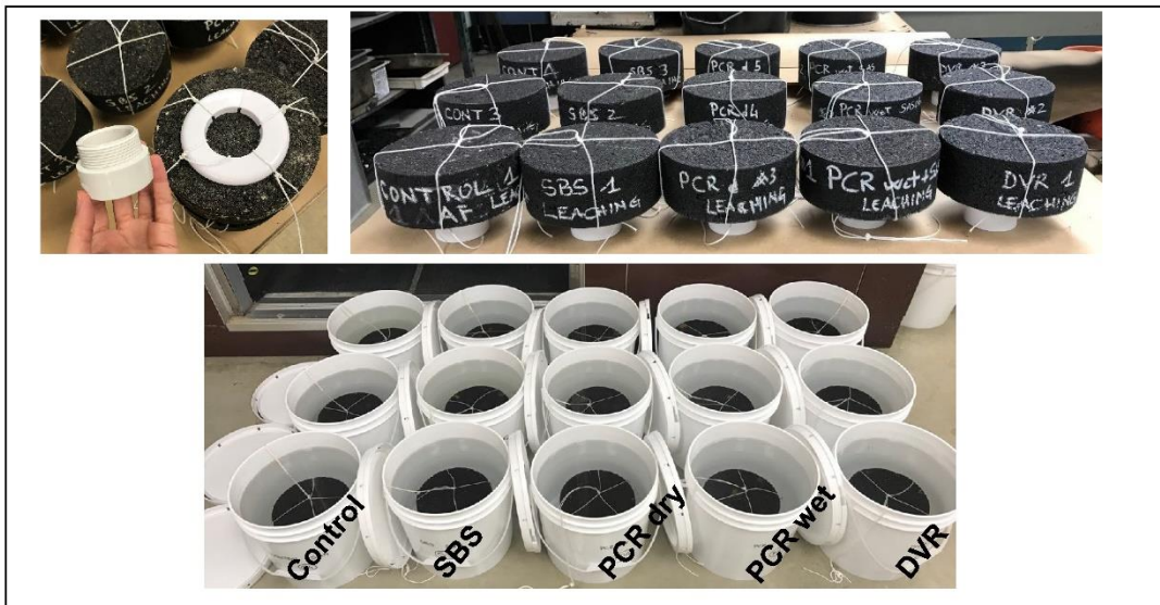
621 Fig 2. Plastic support is attached to the asphalt mix specimens, and specimens are placed in 622 deionized water.
