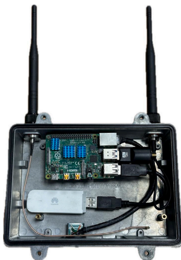
Fig. 3. Hardware solution composed of a Raspberry Pi 4 Model B, a USB WiFi dongle with an external antenna, a USB LTE antenna, all inside an IP67 waterproof box.
