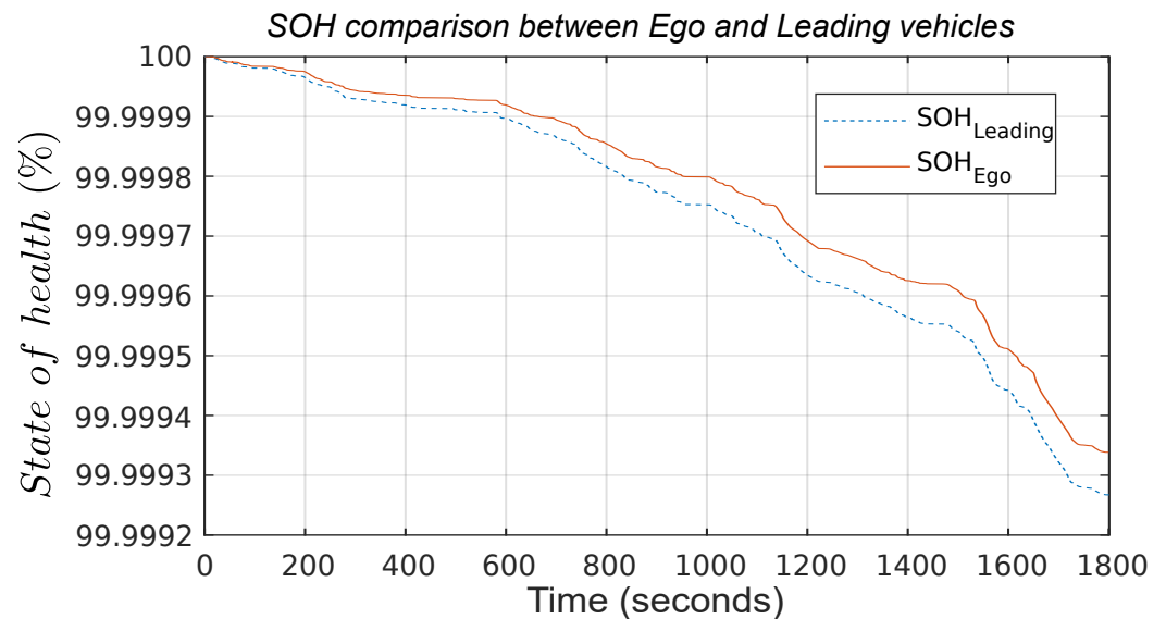
Figure 10. Reduction in battery health degradation due to optimal adaptive cruise control.
