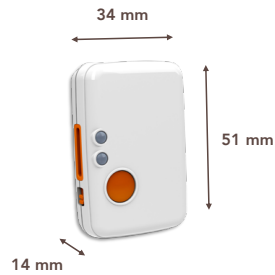
Figure 7.1: Dimensions of the IMU adopted in the study (Shimmer3, adapted from: https://shimmersensing.com/ )
