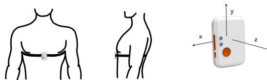
Figure 7.2: Sensor placement adopted in the study, along with the orientation of each axis. In detail: x : medio-lateral, y : axial (longitudinal), z : antero-posterior (vertical)
