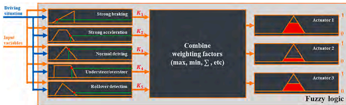
Fig. 12. Simplified diagram of a fuzzy logic CA algorithm.
