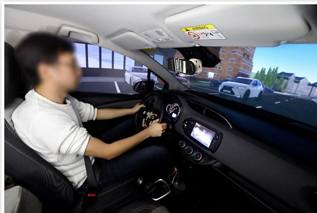
FIGURE 5 Driving simulator (TU Delft Advanced Vehicle Simulator).
