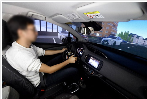
FIGURE 5 Driving simulator (TU Delft Advanced Vehicle Simulator).
