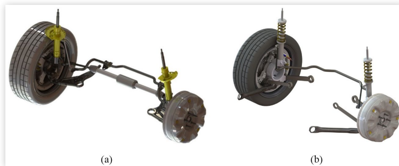
FIGURE 8 Vehicle corners with in-wheel motors on (a) front suspension and (b) rear suspension.
