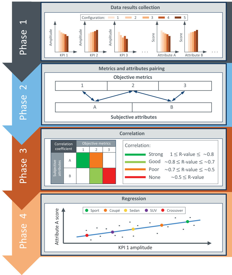
Figure 10. Schematic of the workflow of the subjective-objective correlation process.
