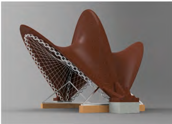
Fig. 12. A rendering showing how the winged pavilion can be used as a centring.
