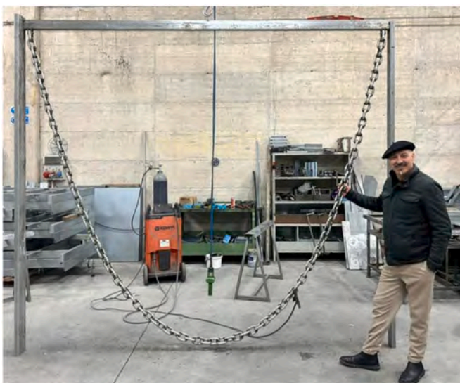
Fig. 5. The hanging chain that has been welded to obtain a catenary frame.
