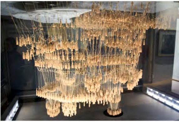
Fig. 1. Gaudi's Hanging Weights Model, picture courtesy eethaannn available at: https://flic.kr/p/2g24Jcm (CC BY-NC 2.0).
