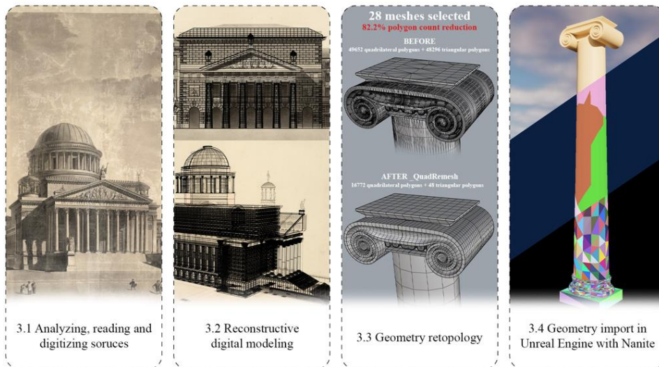
Figure 1. The proposed workflow, from left to right: 3.1: Digitizing sources; 3.2: 3D Modeling; 3.3: Geometry retopology; 3.4: Interoperability between Rhinoceros and Unreal Engine. Source: Vanni, E.
