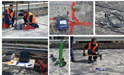
Figure 11. Dynamic identification experimental tests.
