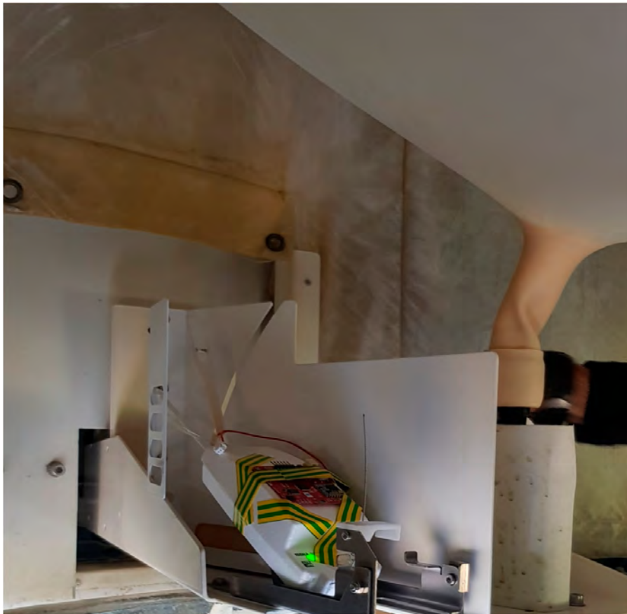
Figure 48: Preparation: attaching cloud walker (COMPLETE) radioprobe to Vaisala RS-41 probe.
