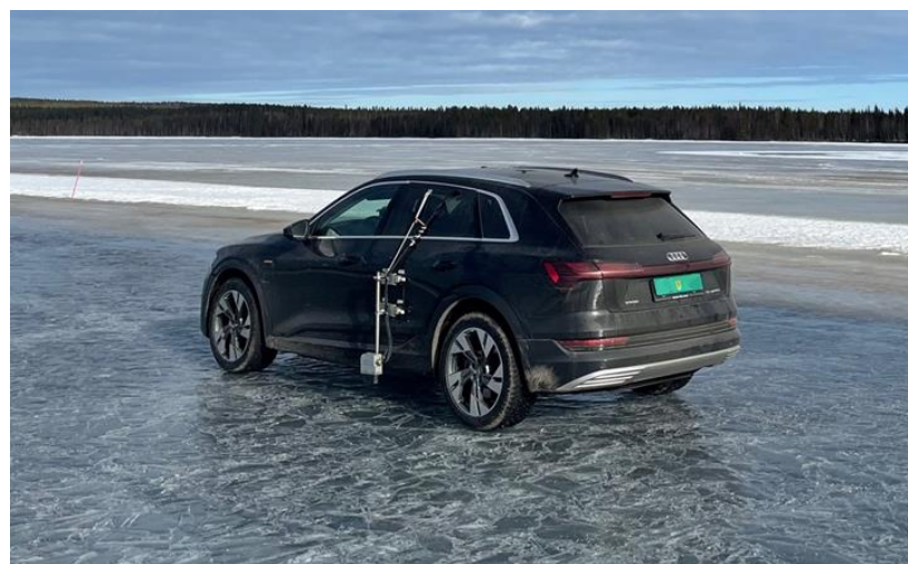
Figure 1. The case study Audi e-tron at the Ebbenjarka testing facility (Sweden), including the Kistler Correvit S-350 sensor, providing accurate measurements of the velocity components.
