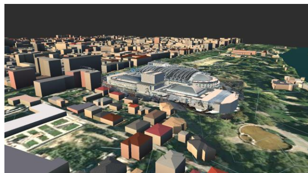
Figure 3. (above) UAV photogrammetric point cloud pertaining to the area of Torino Esposizioni in Turin (below) Lod 400 3D model achieved in manual and time-consuming way for the Torino Esposizioni architectural complex in a CIM view accomplished using Infracworks sw. (Aboohamzeh 2023)
