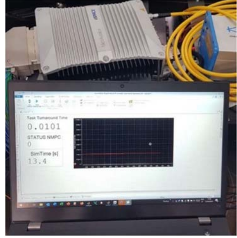
Fig. 6. Real-time implementation of NMPC adv on a dSPACE MicroAutoBox III unit.
