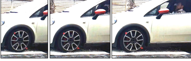
Fig. 14. Image sequence (from left to right) of a production M1 vehicle equipped with its factory-installed ABS, during the extreme high-to-low tire–road friction step test. The red markings on the tire highlight that the wheel does not rotate (i.e., it is locked) in the low- \mu section, represented by the wet white plastic boards (the edge of the white board in the bottom right of each image can be used as a static visual reference).
