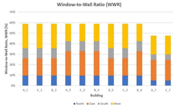
Figure 3: WWR per façade orientation.
