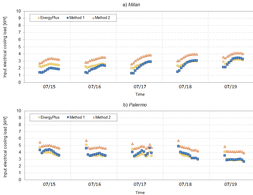
Figure 8. Chiller electrical cooling load in Milan (a), and Palermo (b) on working days of a week in July.
