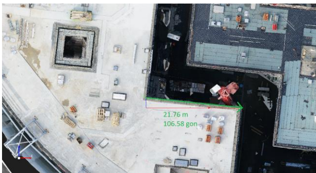
Figure 5. Zoom on generated orthophoto. Distance can be easily computed defining start and end points.
