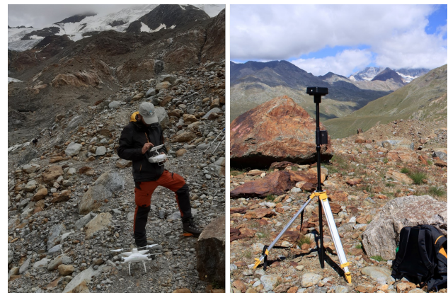
Figure 1. DJI Phantom 4 RTK and D-RTK 2 high precision GNSS mobile station.
