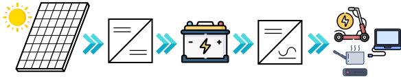
FIGURE 1. Typical power conversion chain of an off-grid PV-storage system supplying local DC or AC loads.
