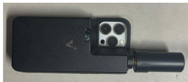
Figure 1. iPhone 15 Pro with the viDoc RTK Rover
